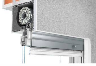
TP1000K shutter built-up from the outside. The external front profile is grooved and equipped with a concealed lath. For better aesthetics, the internal front profile is smooth.
