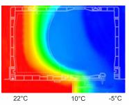
The top mounted roller shutters recommended most frequently by the manufacturers cause keeping the heat inside the building. In the layer between the shutter curtain and the window there is an airbag constituting an excellent insulating layer, i.e. a specific buffer, both for hot and cold air.
