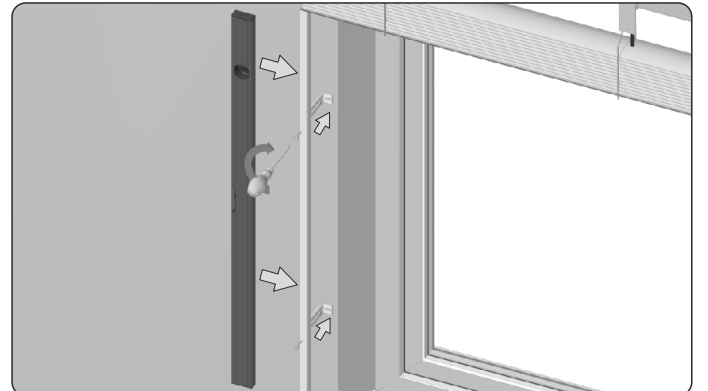
14. Measure the position of the guide axis carefully, then screw the guides to the ground.
