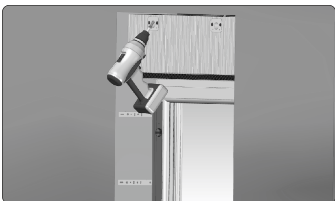
20. The ready set shall be installed in compliance with installation instructions in the earlier made recess. Before final anchoring of the shutters, their vertical and horizontal alignment shall be verified.
