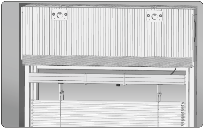
9. Insert the external blinds profile into the box, into the handles of the upper rail.
