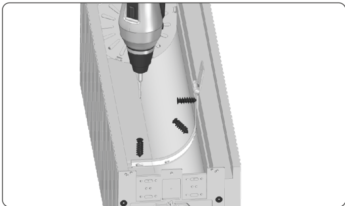
13. Static console shall be fixed to the box by means of plastic fixing screws included in the set.
