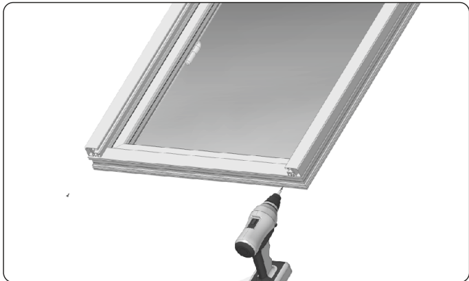
11. Place bottom end caps over the guides and fix them with bolts.
